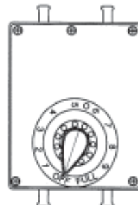
Figure 2-23. Bypass and Control Assembly (BCA)
